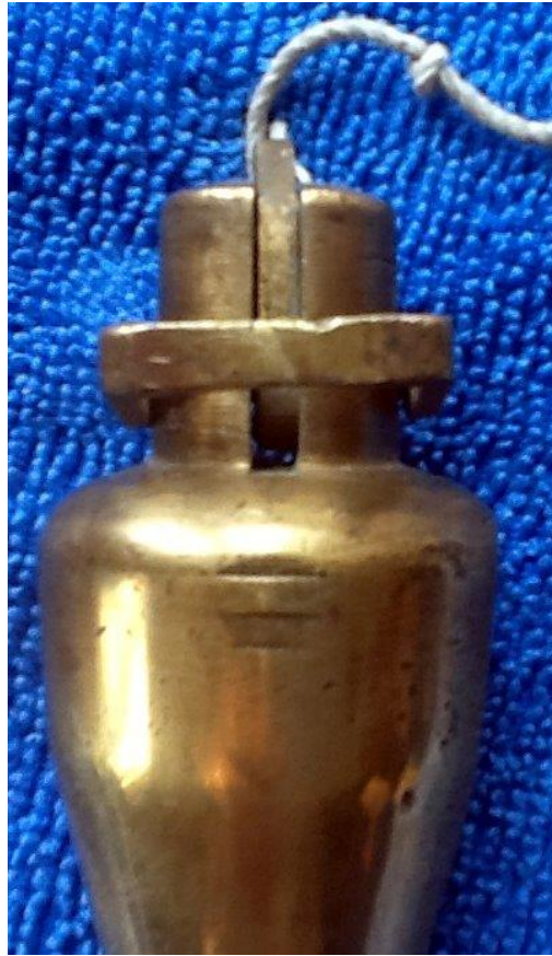
#11 no markings 407 gm. 4 1/2" high 1 1/2" diameter Hinged point. For measuring in oil tanks.
