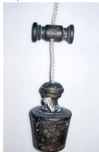
OTTOMAN plumb bob type 4 with spacer
