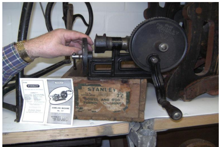
Also more woodworking machines. This is the #77 “dowel and rod turning machine” from Stanley Rule & Level Co (produced 1911 to 1969). More see www.woodmagazine.com
