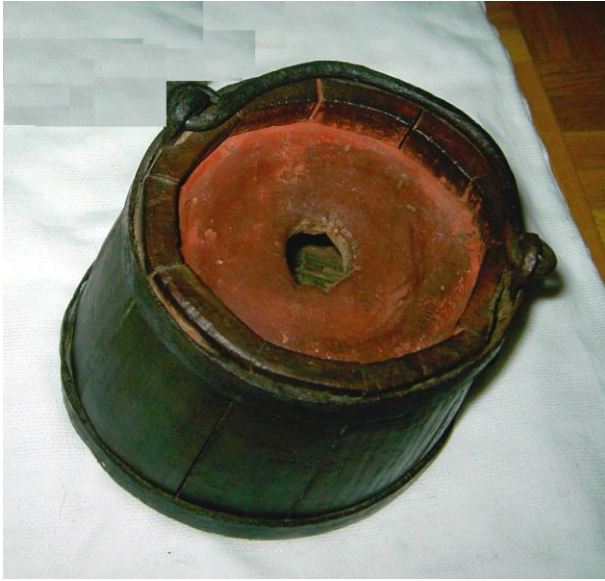
Pot with a red color (Rötel). In Austria the chalk line is also called „Rötelschnur“
