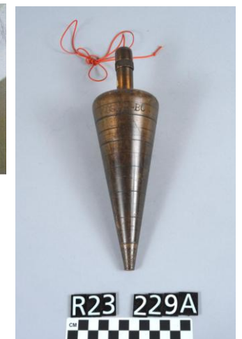
Boulder Canyon. Suspension plumb line in AZ elevator shaft machine room. Used in plumbing observations.
